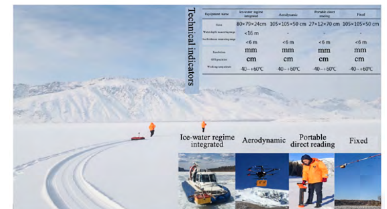
Complete Equipment, Indicators and Applications of Integrated Ice-Water Regime Dual-frequency Radar Measurement
