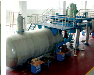
Universal test stand of advanced hydraulic machinery model
