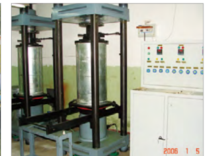
Creep testing system for fully-graded concrete
