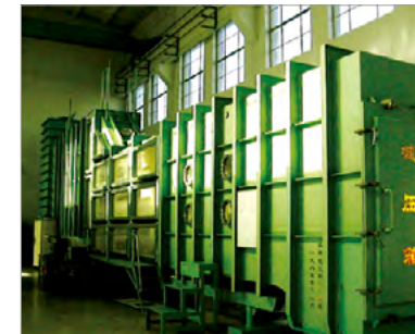
Vacuum tank (vacuum percentage 98.7%; flow discharge 1.0 m³/s)
