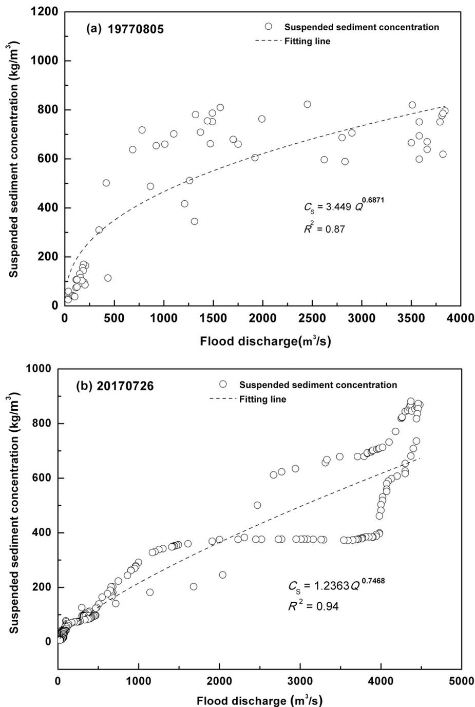
Fig. 4. Sediment rating curve under extreme rainstorm on August 5, 1977 (a) and July 26, 2017 (b) in Wuding River Basin.
