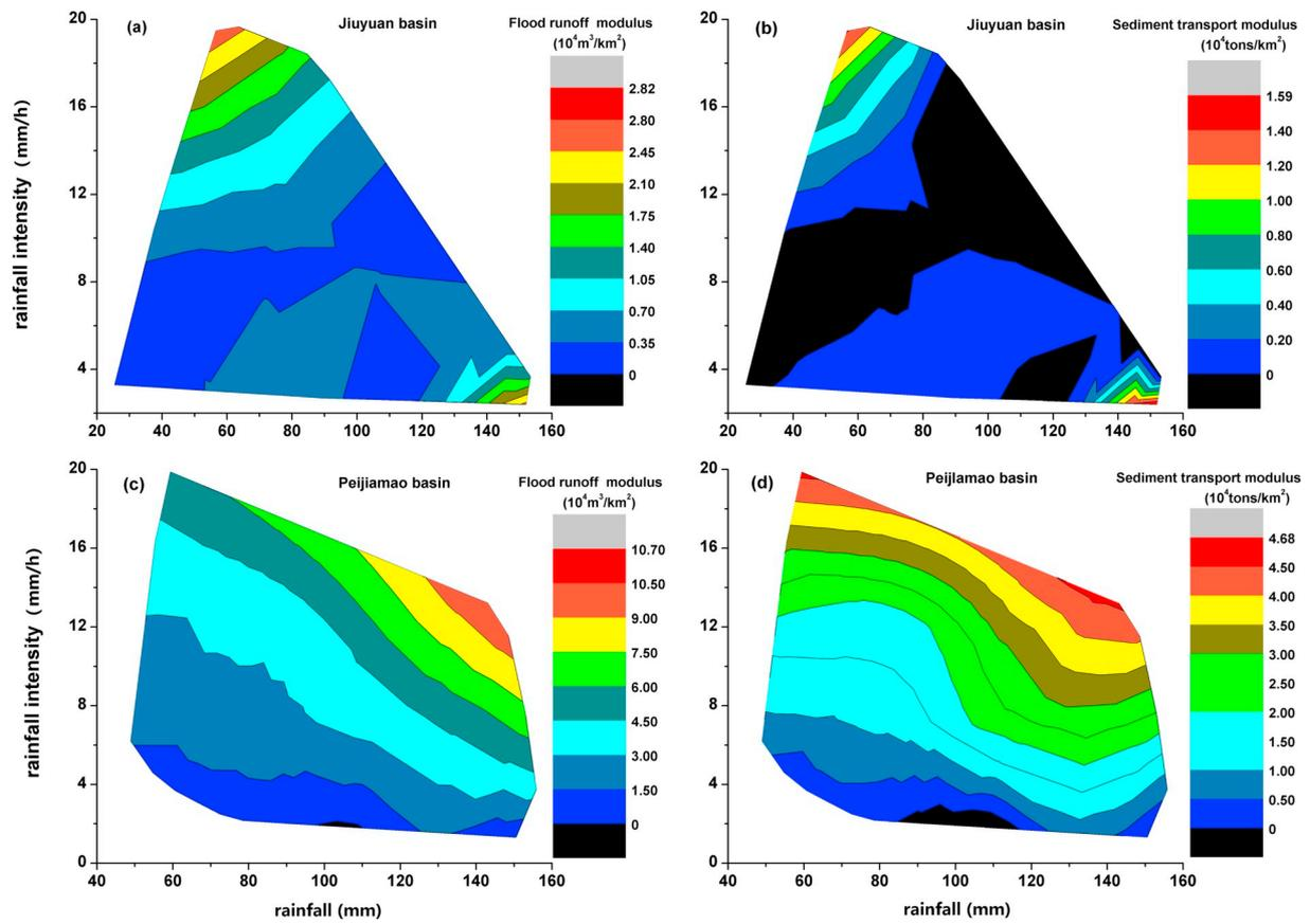
Fig. 6. Contour maps of flood runoff modulus and sediment transport modulus in Jiuyuan Basin (a, b) and Peijiamao Basin (c, d). Here, a two-dimensional (2D) graph was used to present 3D results by using different colors to differentiate between different Z values.
