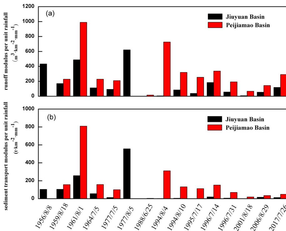
Fig. 7. Runoff modulus per unit rainfall (a) and the sediment transport modulus (b) under similar extreme rainfall conditions in the compared basins.
