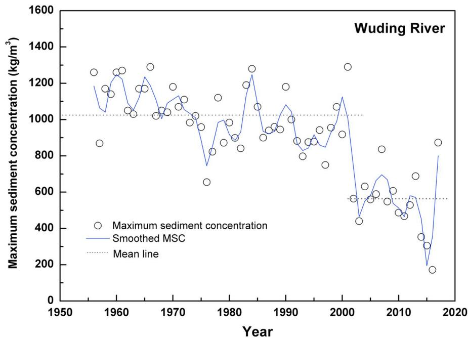
Fig. 3. Maximum suspended sediment concentration of floods changes in the Baijiachuan hydrologic station of Wuding River basin over the years. Here, the gauging station at Baijiachuan was selected as it is located at the outlet of the Wuding River basin.
