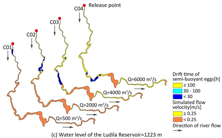
Fig. 5. Final states of semi-buoyant eggs in different scenarios. (For interpretation of the references to color in this figure, the reader is referred to the web version of this article.)
