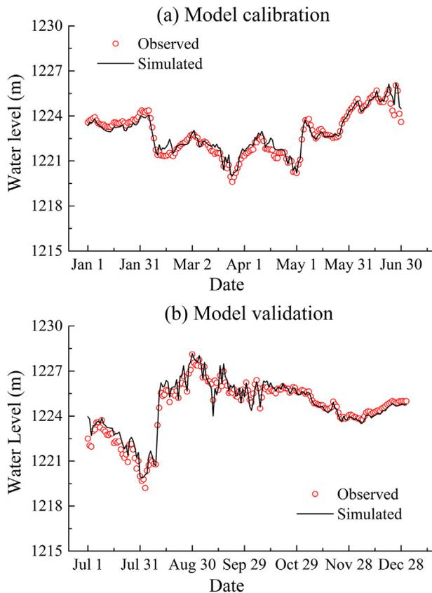
Fig. 3. Simulated and observed water levels at Zhongjiang station (2015).
