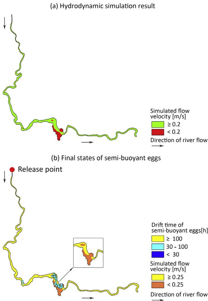
Fig. 6. Hydrodynamic simulation results and final states of semi-buoyant eggs. (WL = 1223 m, Q = 15,000 m<sup>3</sup>/s).
